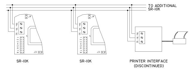
Set each interface to unique address. Install RS-485 termination jumper, J4, on the first and last units only.
